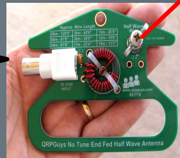
Matching Unit 49:1 Transformer
