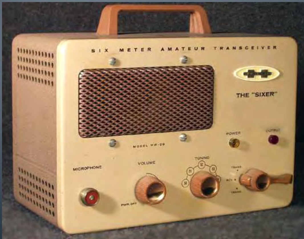
Benton Harbor Lunch Boxes — Complete Transceivers . . . for 6 and 2 meters. Feature crystal-controlled transmitters with 5-watt input and tunable super-regenerative receivers with RF stage. Built-in 115 VAC power supply and speaker. Mike included. Less crystal. Kit HW-29A, 6-meter, 9 lbs., no money dn., $5 mo. $44.95 Kit HW-30, 2-meter, 9 lbs., no money dn., $5 mo. $44.95 Kit GP-11, Mobile Vibrator Power Supply, 6 lbs. . . $17.95
