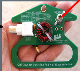
Matching Unit 49:1 Transformer
