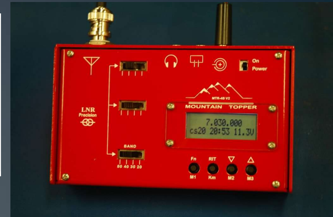
LNR Precision MTR-4B ver 2.3 $350 5 to 13 V 27 mA RX
