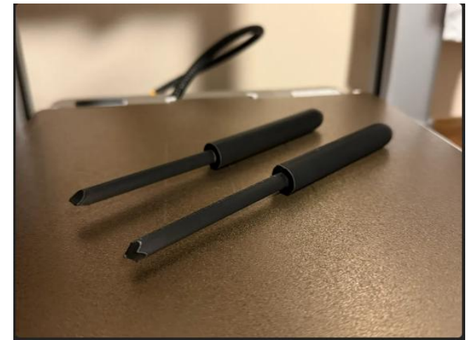
Non-conductive tools help in RF circuit alignments.
