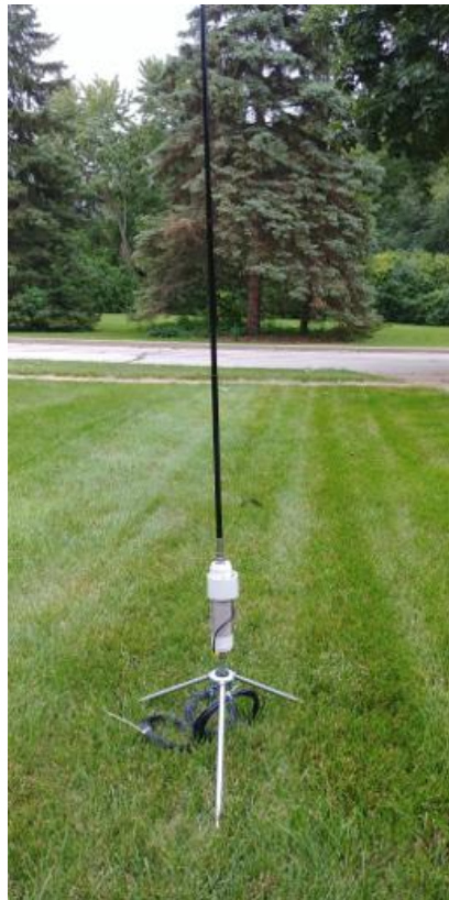
Wolf River Coil Take It Along 1000 80 to 10m Collapsible 102" Whip Three 33' radials Footprint: 19" x 17" Wt: 3 lb 5 oz
