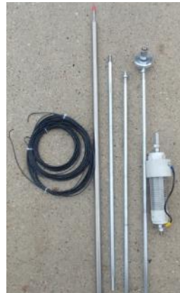
Wolf River Coil Take It Along 1000 80 to 10m Collapsible 102" Whip Three 33' radials Footprint: 19" x 17" Wt: 3 lb 5 oz
